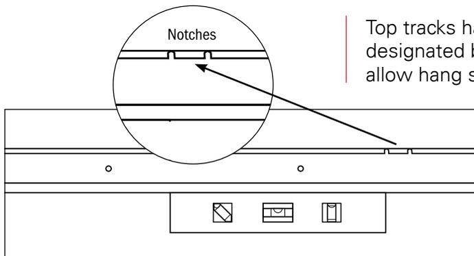
Top tracks have a top and a bottom. The TOP is designated by a label and has two notches to allow hang standards to be inserted properly.
