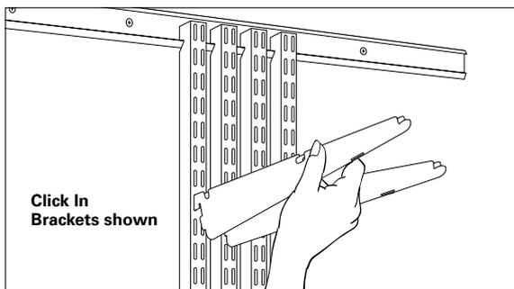
1. Group hang standards together and insert bracket click in at the appropriate height based on your space plan.
